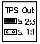
GTS-GTR ECUs that have a bottom PCB version of 1.2 onwards also have a jumper for setting the scale of TPS Out. The ECU sends the TPS signal to the Automatic Transmission Controller and 4WD Controller.
